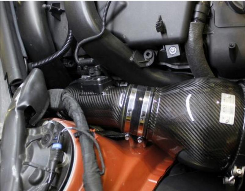
36. Finally – reconnect the MAF sensor plug – there should be enough slack in the loom from removing it from the clip earlier. Ensure the connector is clicked in all the way.
