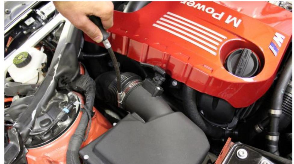
4. Loosen hose clamp on the left side (looking at the engine) airbox.
