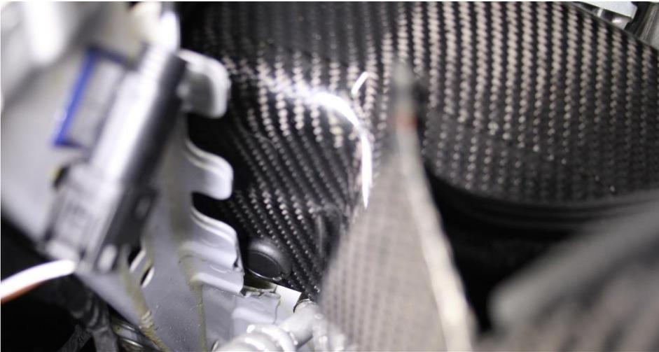
24. Now do the same with the other side. You will need to push the duct away from the chassis metal work to get access to the hole. Once secured – you will notice that the duct still has some movement – this is required for allowing adjustment on the intake housing.
