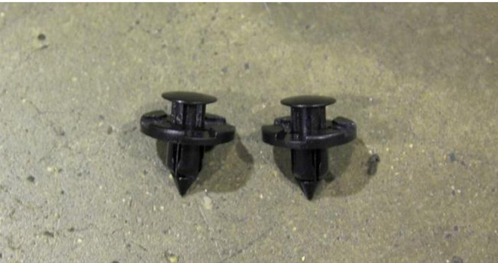
55. Using one of the smaller push rivets supplied, insert into the aligned bracket and lock into place by fully pushing in the head as shown next.
