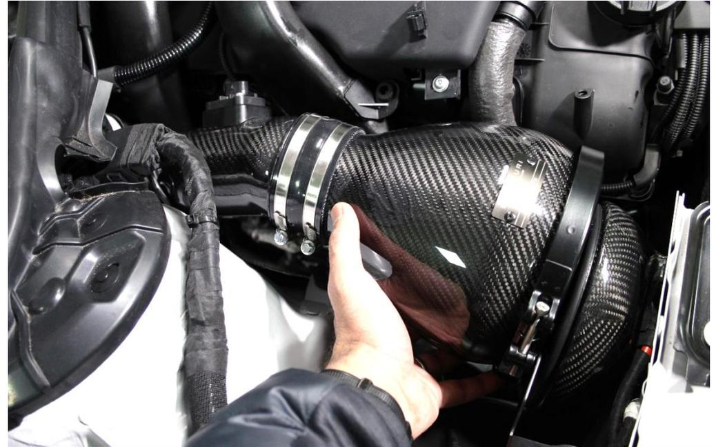
33. Lower the intake assembly into the left side and push the tube into the silicon coupler installed previously. Locate the opening of the intake into the duct installed previously
