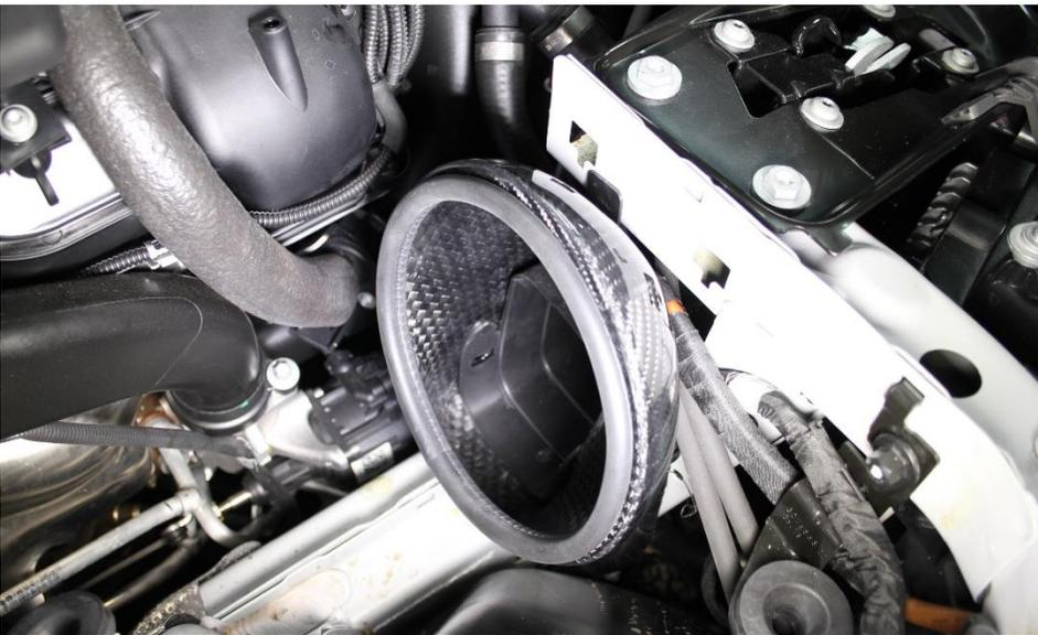
26. Locate the left duct onto the stock opening. The stock plastic opening should go INSIDE the new duct.
