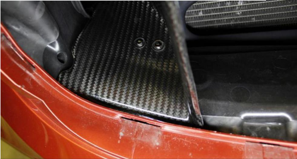
53. Now pull the bumper area at the bottom of the grill out to allow the lower lip of the scoop to locate underneath.
