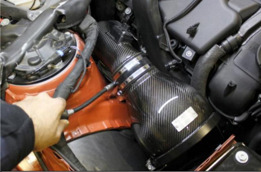
35. Now tighten the clamp on the tube as shown – ensure there is no gap between the flange on the tube and the silicon.
