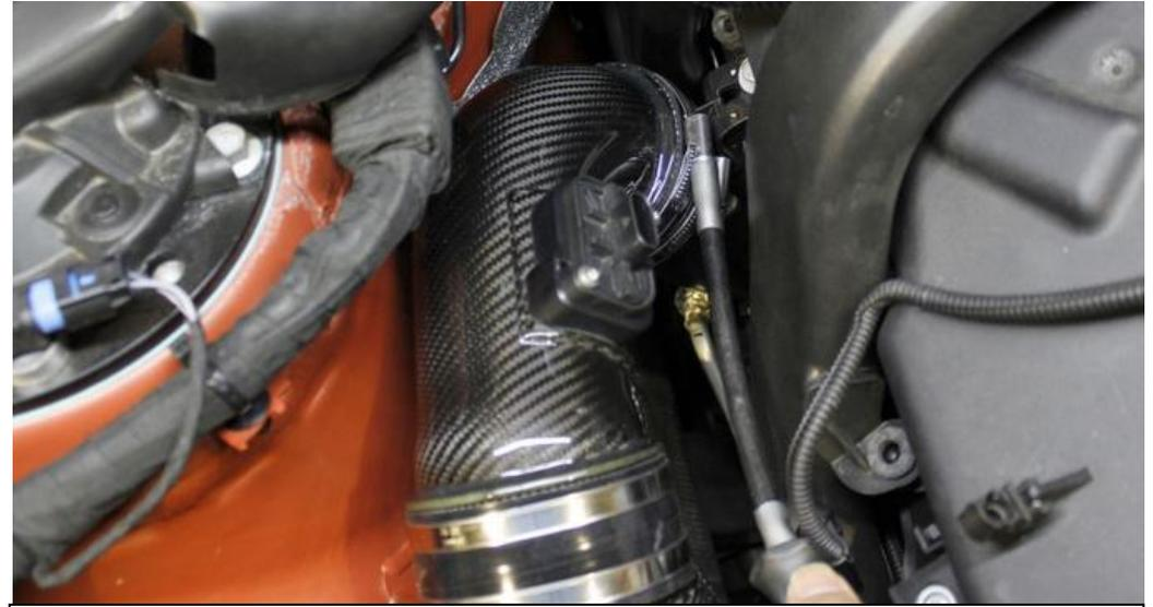
35. Now tighten the lower clamp on the tube – ensure there is no gap between the flange on the carbon tube and the silicon. **MAKE SURE THIS CLAMP IS CLOSE TO THE CARBON TUBE AND STRAIGHT ALL THE WAY AROUND.**
