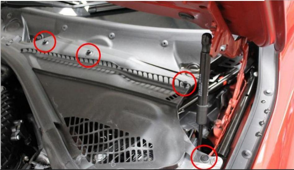
1. Remove the two plastic panels at the back of the engine bay by removing the plastic tab and rotating the 3 plastic nuts 90 degrees.
