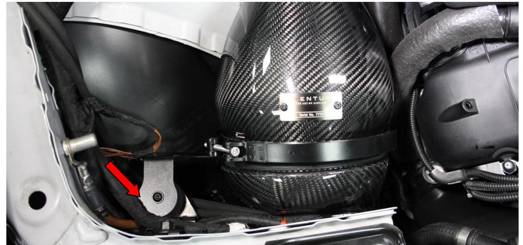
35. Push the boss on the mounting bracket into the stock rubber grommet fully. Ensure the housing is positioned evenly into the seal of the duct.
