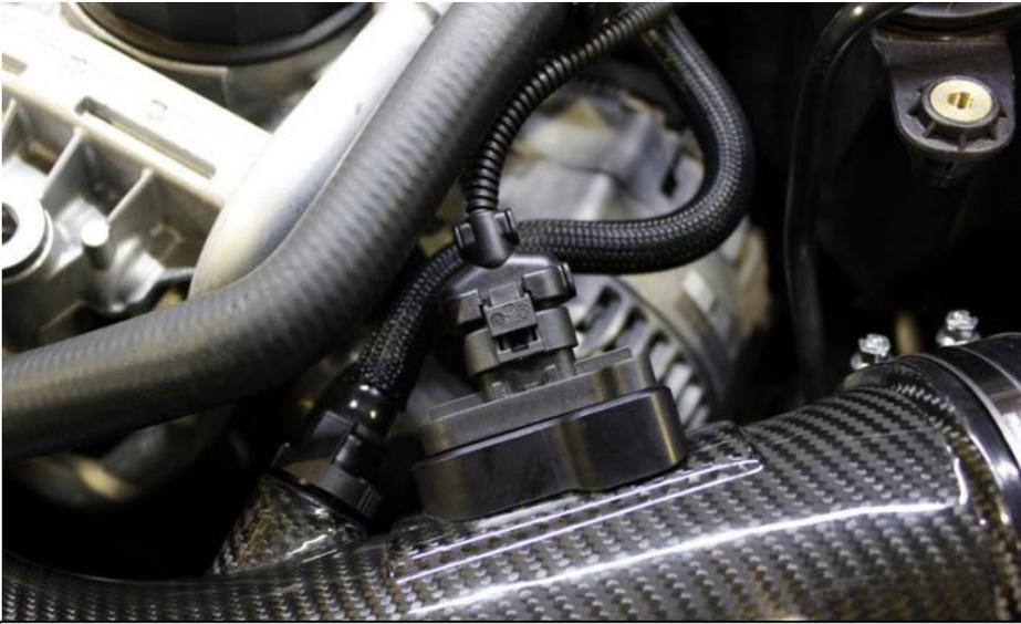
43. Insert breather tube into place – it should click into place. Reconnect MAF sensor plug ensuring it has engaged fully.
