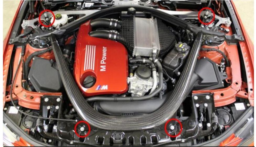
2. Remove the 8 13mm bolts holding the strut brace down. There is also a 10mm bolt secured to the coolant tank – see next photo.
