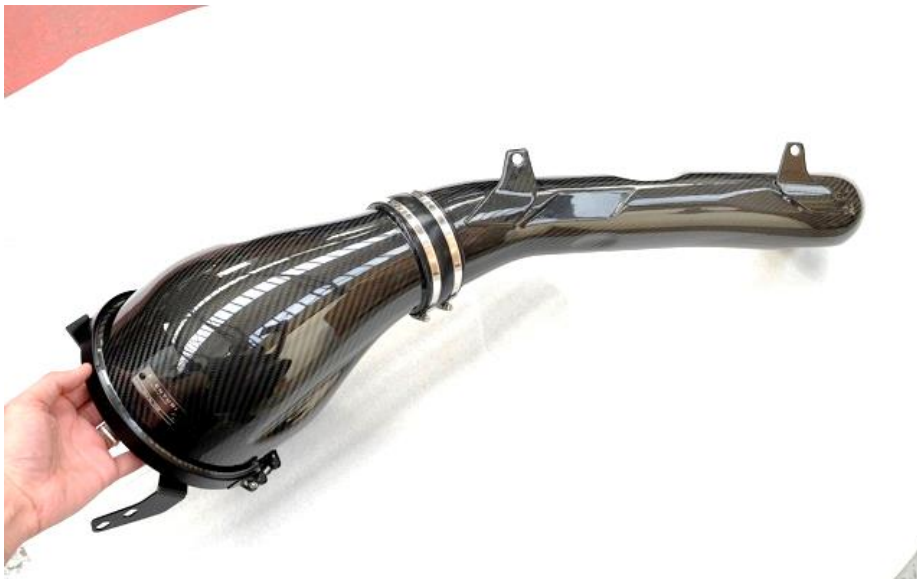
34. Another angle of the housing and tube. Leave the clamps loose to allow the housing to be rotated.
