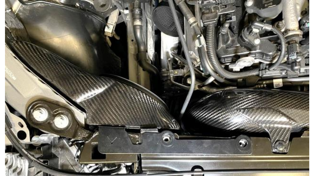
51. Position the duct so the bracket lines up with the 2 holes. Or single hole for the updated version.
