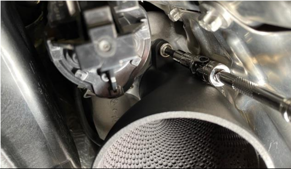
48. Insert the remaining Torx screw in the top hole and tighten. We recommend using a magnetic socket or another means to secure the screw to the Torx bit while inserting.
