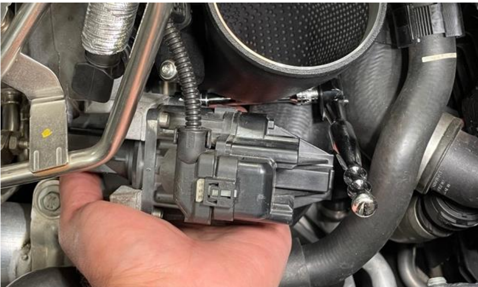
22. Once the screw has caught the thread - use a ratchet to tighten - again you can support the extension as shown. Tighten to 15Nm.
