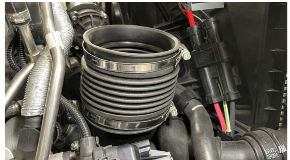
27. Position 2 x 80-100mm hose clamps as shown and tighten the lower one around the inlet. Do not over tighten.
