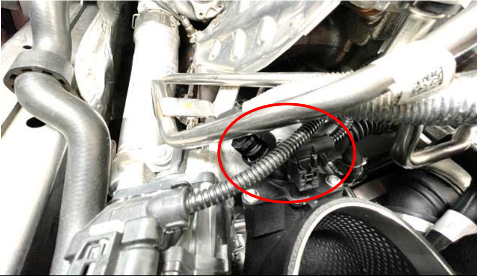
17. Reconnect the sensor plug and the breather tube.
