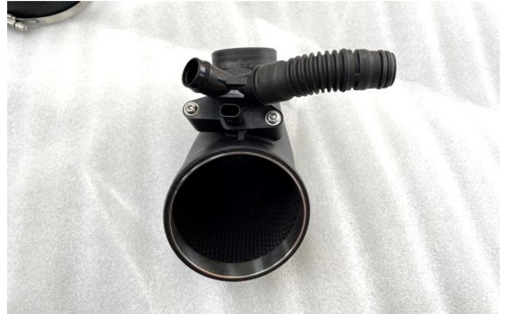
14. Secure the breather assembly onto the inlet using the OEM screws. If the O-ring on the breather is too thick – please replace it with the one supplied in the kit.
