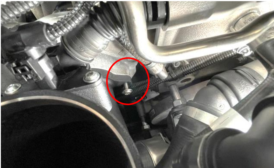
19. Line up the inlet and use one screw on the right side - turn it by hand to ensure you do not cross thread the turbo. DO NOT fully secure yet - leave it loose.
