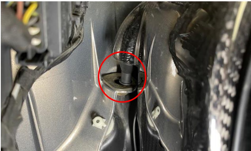
30. The back of the carbon duct secures into the OEM rubber grommet shown. Push the mount into the grommet.
