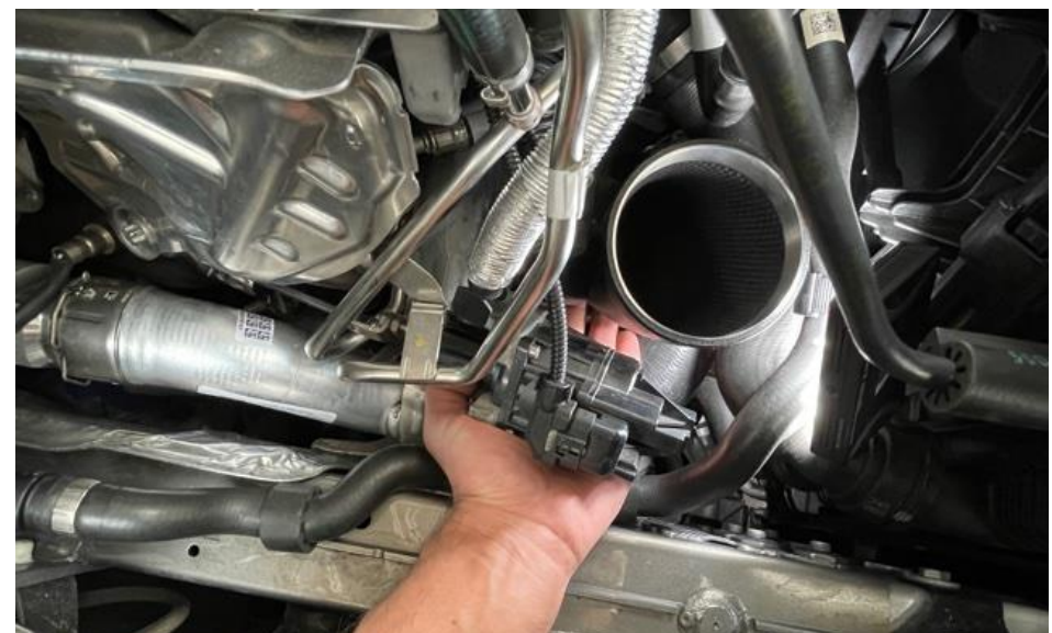
19b. The other side is more tricky to get to - you can reach under the turbo module as shown to support the screw on this side and get it into place.
