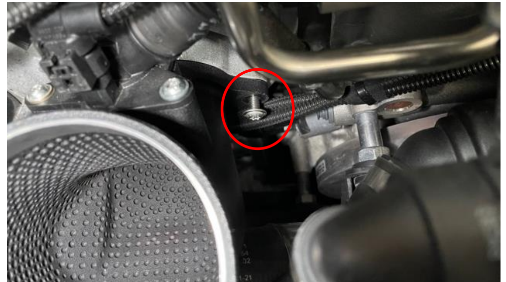
23. Now secure the right side screw to 15Nm.
