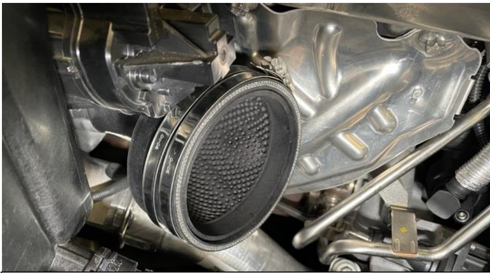
54. Take the remaining silicon hose and 2 x 90-110 clamps. Push the silicon all the way over the inlet - you need space to drop the filter housing into place.
