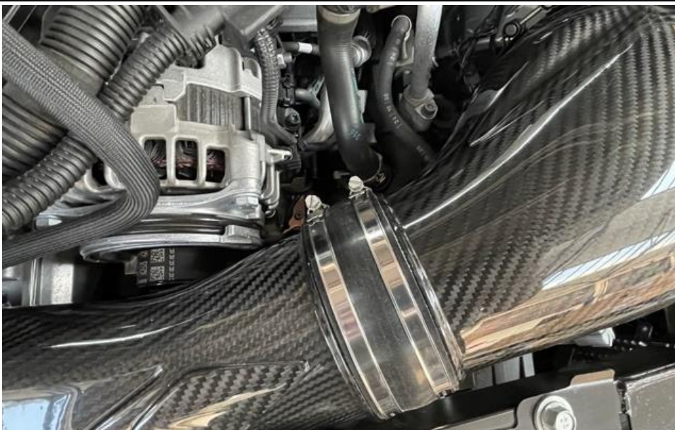
42. Tighten the hose clamps around the tube and housing - do not overtighten otherwise you can damage the carbon.
