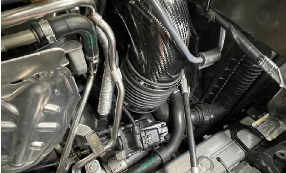
40. Tighten the clamps - do not overtighten otherwise you can damage the carbon.
