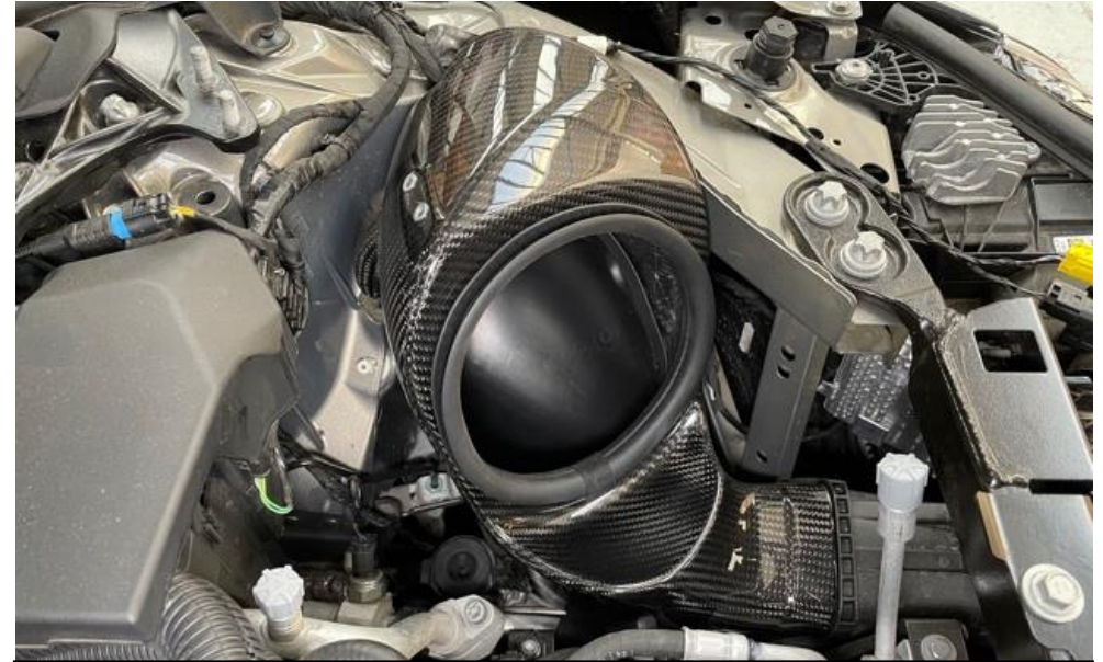
29. Lower the duct into place - it should connect to the OEM air duct as shown.
