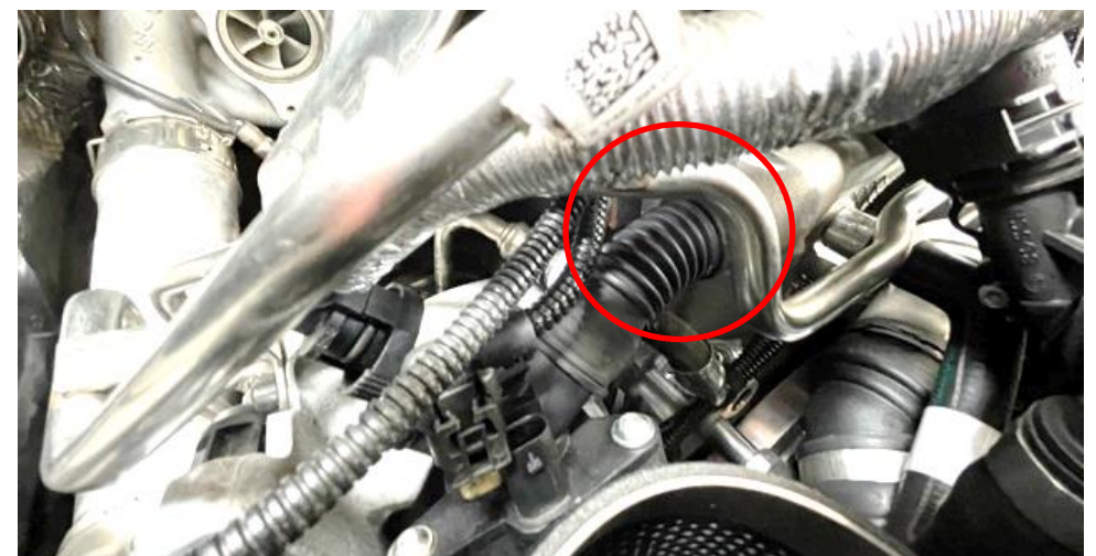
16. Push the breather back into place and secure with the clip. Push the inlet into the turbo fully.
