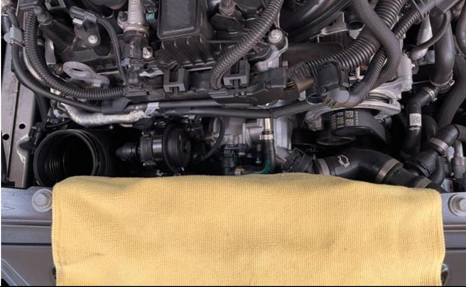
32. Cover the metal tabs with a cloth to protect the carbon tube.
