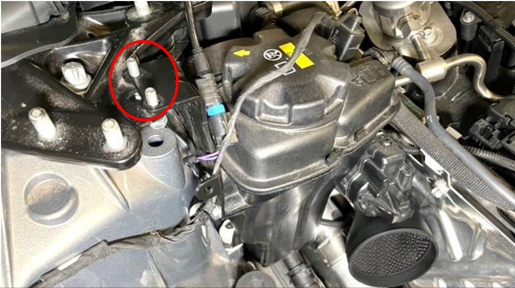
52. For more clearance we now need to move the coolant tank. Remove the 2 x 10mm nuts on the coolant bracket shown.
