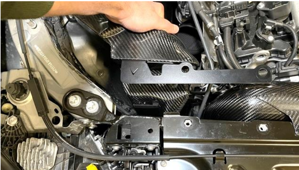
50. Lower the LHS carbon duct into position. The bracket will sit on top of the slam panel where the screws were removed.
