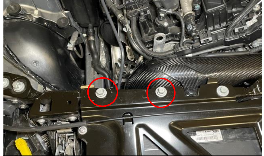
49. Remove these 2 bolts. If you have the updated intake you only need to remove the left most one. Check the bracket on top of the LHS duct to see how many holes it has.
