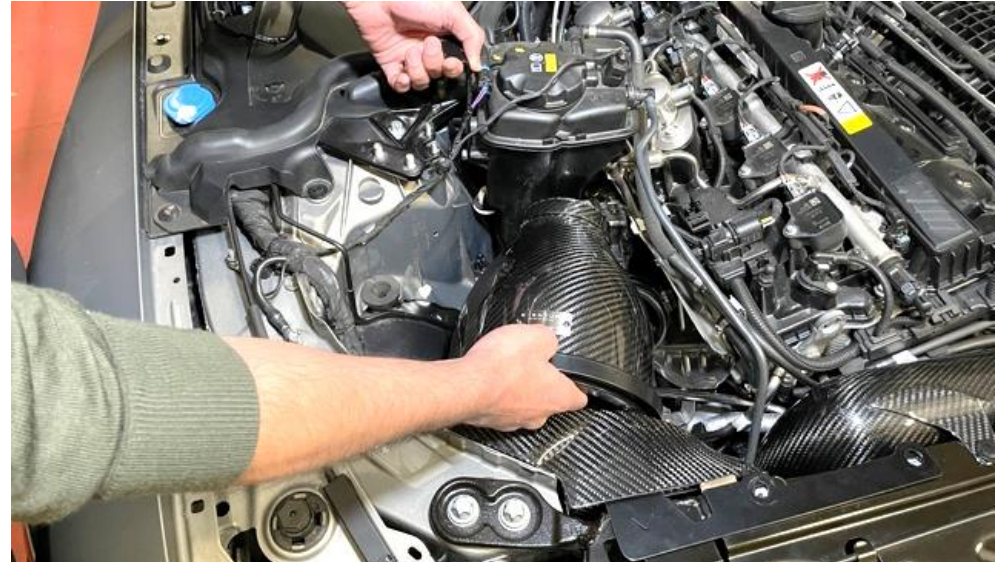
55. Lift the coolant tank and lower the LHS housing down.
