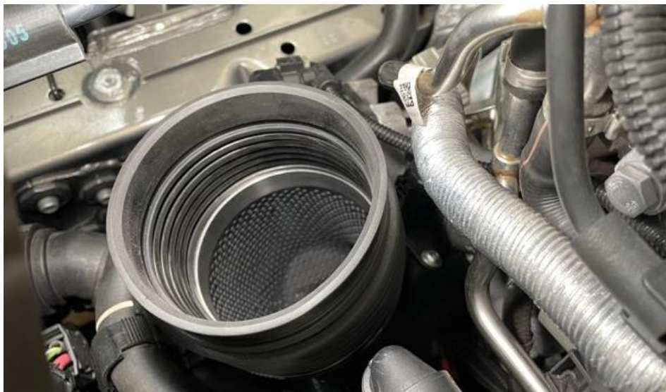
26. Push the hose onto the inlet making sure the TOP stays on top. Push it down fully so the inlet ends where the flexible portion starts.
