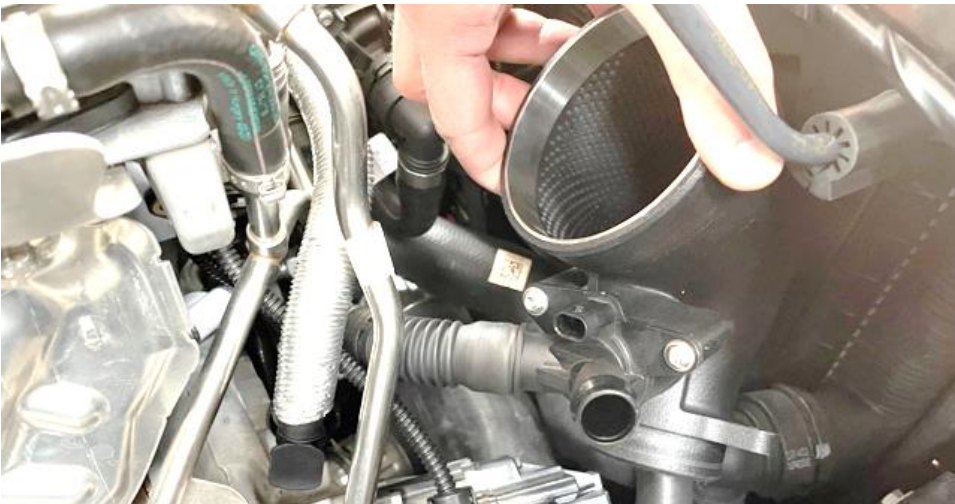
15. Lower the inlet into place - the breather needs to go back into the engine as the inlet is positioned.
