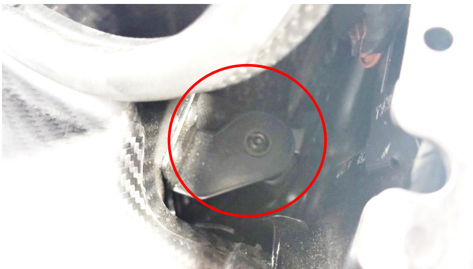
19. There is also a second mount towards the front of the car – ensure that is correctly pushed in.
