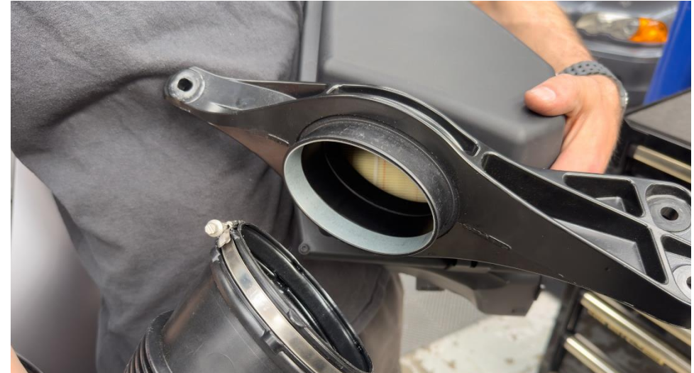
8. Remove the flexible hose from the airbox and you can now remove the strut brace.
