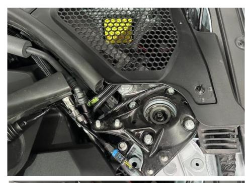
4. If the rear studs do not line up with the brace you will need to adjust the brackets around the strut supports on each side. Adjusting these will not affect vehicle alignment. Remove the trim covers over each strut.
