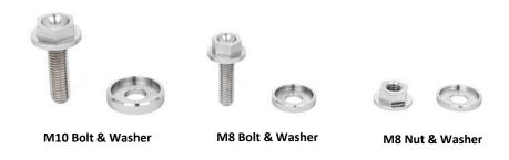
2. The new Eventuri brace comes with its own hardware. The washers are specific to the bolts and nuts. The washers for the M8 bolts will not fit the nuts. They have different thicknesses and widths. Please do not mix them.
