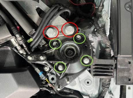
5. Ensure the car is fully on the ground. Loosen the 21mm (red) and the E14 bolts (Green). You don't need to remove them. The support bracket with the studs will now have some movement.
